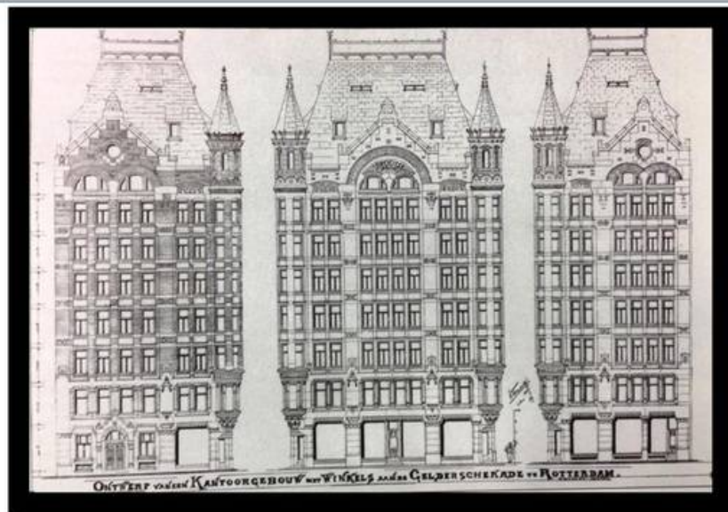
Figure 6: Façade plan of the ( Witte Huis ) 'white house' in Rotterdam. This plan shows the north view (right of picture), east view (middle of picture) and south view (left of picture) (Photograph by Damen, Camp, Devolder, 1991).
