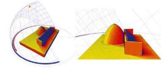
Figure 6. 3D models of Khaju Bridge with solar analyses, the facade of Khaju Bridge protects the water pond from the deleterious effects of the sun and wind. Research shows that during the winter time the pond does not receive any direct sunlight which can mean ice forming in cooler temperatures above 0°C. (Hensel, Gharleghi, Craig, Hensel, 2012) (photograph by Hensel, Gharleghi, Craig, Hensel, 2012).
