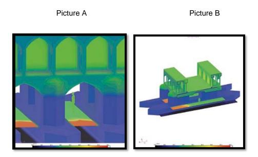
Figure 5. Picture A shows an axonometric of the bridge and Picture B shows the section of Khaju Bridge. Analyses of heat transfer shows that surface temperature of Khaju Bridge during the summer time is cool owing to the fact that the special design of the structure brings about a comfortable environment on this bridge. (Hensel, Gharleghi, Craig, Hensel, 2012) (photograph by Hensel, Gharleghi, Craig, Hensel, 2012).
