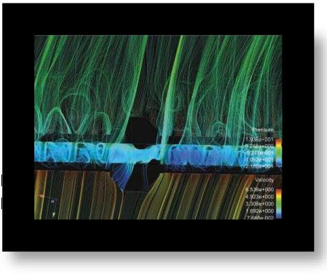
Figure 11. Analysis showing that the evenly spaced arches in this structure change the wind speed bringing a low breeze (3.2 kilometres per second) onto the roadway. This means that the structure brings about a comfortable environment along the path (Hensel, Gharleghi, Craig, Hensel, 2012) (photograph by Hensel, Gharleghi,-Craig, Hensel, 2012).
